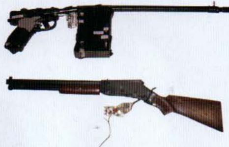
It took less than a year for lightguns to be integrated into the project, and only one prototype (right) to reach a handsome, realistic replica rifle (below left). By December 1967 the quiz lightgun (above left) was ready. A descendent of the project's first peripheral, the lightpen, it worked by reading the number of dots that made up the spot which corresponded to each answer of the quiz: odd numbers were wrong, even numbers were right
